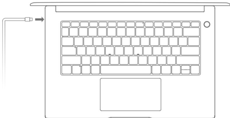
Your computer has a built-in rechargeable battery, and you can charge it using the adapter and USB-C charging cable that came with it. The indicator blinks white during charging.
